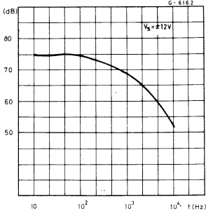
Fig. 6 - Supply voltage rejection vs. frequency
